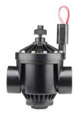
Brand: Landscape Irrigation Product Line: Valves Product Model: 1<sup>1</sup>/<sub>2</sub>" and 2" PGV SKU: PGV201B Description: PGV Valve, screw-top, 2" (50 mm) BSP combination globe / angle valve with flow control and female thread inlet / outlet Weight: 2.7792 UPC-A: 0611698111642 Qty. / Bag: 8 Master Carton: 8 Land Pallet: 336 Ocean Pallet: 384 Origin: Made in Mexico Feature Options: Flow control Inlet Size: 2" Material: Plastic
