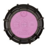
Brand: Landscape Irrigation Product Line: Rotors Product Model: PGP® Ultra & I-20 PRB SKU: I2004SSRPRB Description: I-20 Rotor, 10 cm, adjustable from 50° to 360°, ¾" inlet, stainless steel riser, check valve, reclaimed ID, pressure-regulated body Pop-up Height: 4" UPC-A: 0611698060193 Qty. / Bag: 20 Master Carton: 20 Land Pallet: 1260 Ocean Pallet: 1620 Application Type: Commercial Residential Feature Options: Check valve Reclaimed water Stainless steel Inlet Size: ¾"
