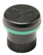
Brand: Landscape Irrigation Product Line: Nozzles Product Model: Bubblers & Bubbler Nozzles SKU: MSBN50Q Description: Multi-Stream Bubbler Nozzle, pressure-compensating, 1.9 l/min, 90°, female thread UPC-A: 0611698144503 Qty. / Bag: 25/250 Master Carton: 250 Land Pallet: 40000 Ocean Pallet: 48000 Application Type: Trees and shrubs Arc: **90**⁰ Nozzle Type: Bubbler Fixed Arc Spec Nozzle Type: Multi-stream
