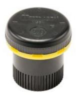
Brand: Landscape Irrigation Product Line: Nozzles Product Model: Bubblers & Bubbler Nozzles SKU: MSBN20F Description: Multi-Stream Bubbler Nozzle, pressure-compensating, 7.6 l/min, 360°, female thread UPC-A: 0611698135839 Qty. / Bag: 25/250 Master Carton: 250 Land Pallet: 40000 Ocean Pallet: 48000 Application Type: Trees and shrubs Arc: 360º Nozzle Type: Bubbler Fixed Arc Spec Nozzle Type: Multi-stream
