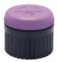
Brand: Landscape Irrigation Product Line: Nozzles Product Model: Bubblers & Bubbler Nozzles SKU: PCB25R Description: Pressure-Compensating Bubbler, flood pattern, 0.9 I/min, ½" thread, reclaimed water ID UPC-A: 0611698145883 Qty. / Bag: 25/250 Master Carton: 250 Land Pallet: 40000 Ocean Pallet: 48000 Application Type: Trees and shrubs Feature Options: Reclaimed water Nozzle Type: Bubbler Fixed Arc Spec Nozzle Type: Bubbler nozzle
