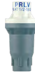
PRLV - Pressure-Regulating Limit Valve Wide-Range Flow Width: 6.4 cm Length: 14.7 cm ¾" FNPT inlet x ¾" FNPT outlet
