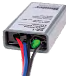
EZ-1 single-station decoder with status LED
