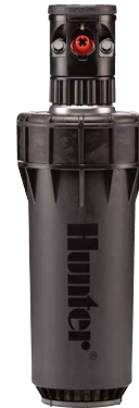
I80-04-SS Pop-up I80-04-SS-ON Pop-up Overall height: 25 cm Pop-up height: 9.5 cm Exposed diameter: 11 cm Inlet size: 1" and 1½"
