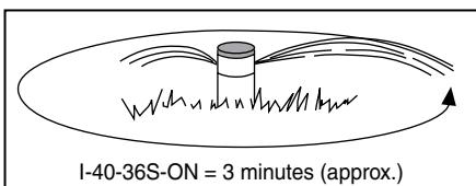
Data represent test results in zero wind. Adjust for local conditions. Radius may be reduced up to 25% with adjustment screw (this may alter the uniformity of the spray pattern).
