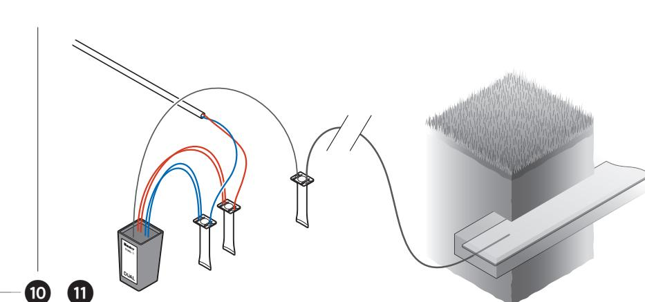
**EN** Connect the earth ground hardware (plate or rod) with the bare copper lead. Use a quality waterproof connector or metal clamp. Use either 4"/100 mm x 36"/1m copper plate, or 8'/2.5 m copper clad steel rod.
