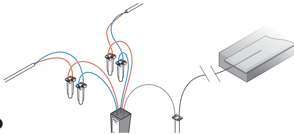
**EN** The surge arrester is installed in-line with the two-wire path, with a red and blue pair of wires on each side, for insertion in the path.
