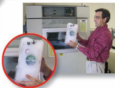
Right: Repetitive heating and freezing cycles in Hunter's Environmental Test Chamber (controllers are tested at extremes ranging from freezing to 96°C).
