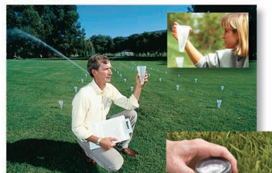
Water audits give a good analysis of an irrigation system's effectiveness through measuring pressure at each sprinkler head and distribution uniformity between heads.
