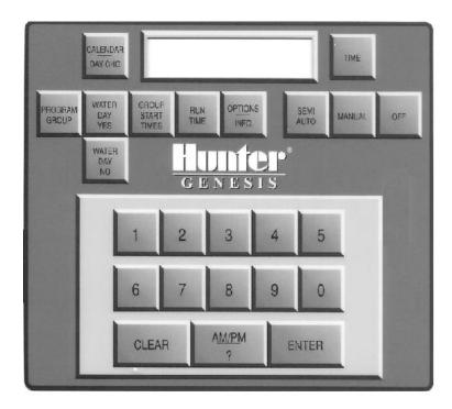
This is the keyboard and display of a typical Genesis Controller. The rectangular window at the top displays messages and other information about the operation of the controller. The keys in the top portion affect programming functions such as Start times, Run Times, schedule, and so on. The keys in the bottom portion are used mostly for data entry.
