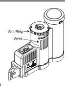
the vent will speed up the dry out time and closing the vents will slow down the dry out time.
