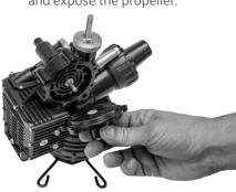
3. Remove the propeller from the housing to clear any debris that may be trapped inside.
