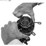
For 360° operation, remove both adjustment rings.
